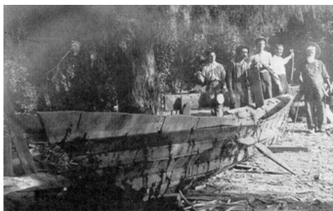
Photo: Replica of a sewn-plank Chumash tomol constructed by J.P. Harrington in 1912. Photo from Terry Jones.
